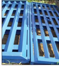
Angled crossbars cause vibration that removes loose tire debris.
