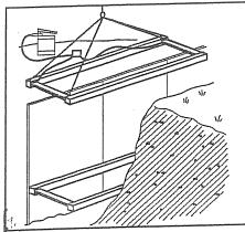
7. Lower the Waler into the excavation in its proper position. (Remember to space the Waler according to the Manufacturers Tabulated Data.)
